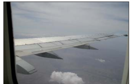
(b) Flaps retracted (cruising)
